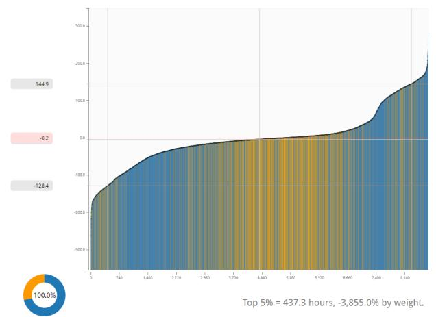
At City Hall shown above, in 5% of the hours at either end of the chart, we see swings of about 120kW from one hour to the next. That leaves 90% of the cases where swings are less than this amount. As expected, swings are far less prevalent on weekends (orange).
