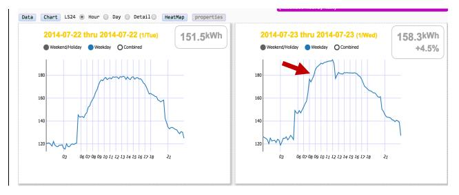
We believe that this load change of approximately 200 kW (5 minute kWh pulses x 12) is the result of turning on/off the final stage of cooling.
